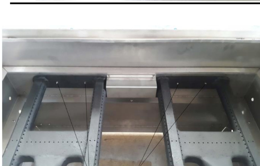
Pop Rivets to loosen gas burners
