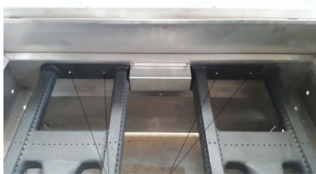
Pop Rivets to loosen gas burners
