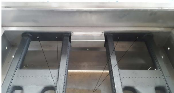
Pop Rivets to loosen gas burners
